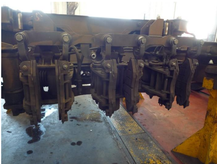
Figure 2-1: Brake pads at bogie
